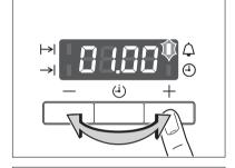
After approx. 5 seconds the display shows the time remaining. The function indicator Countdown (a) lights up.
